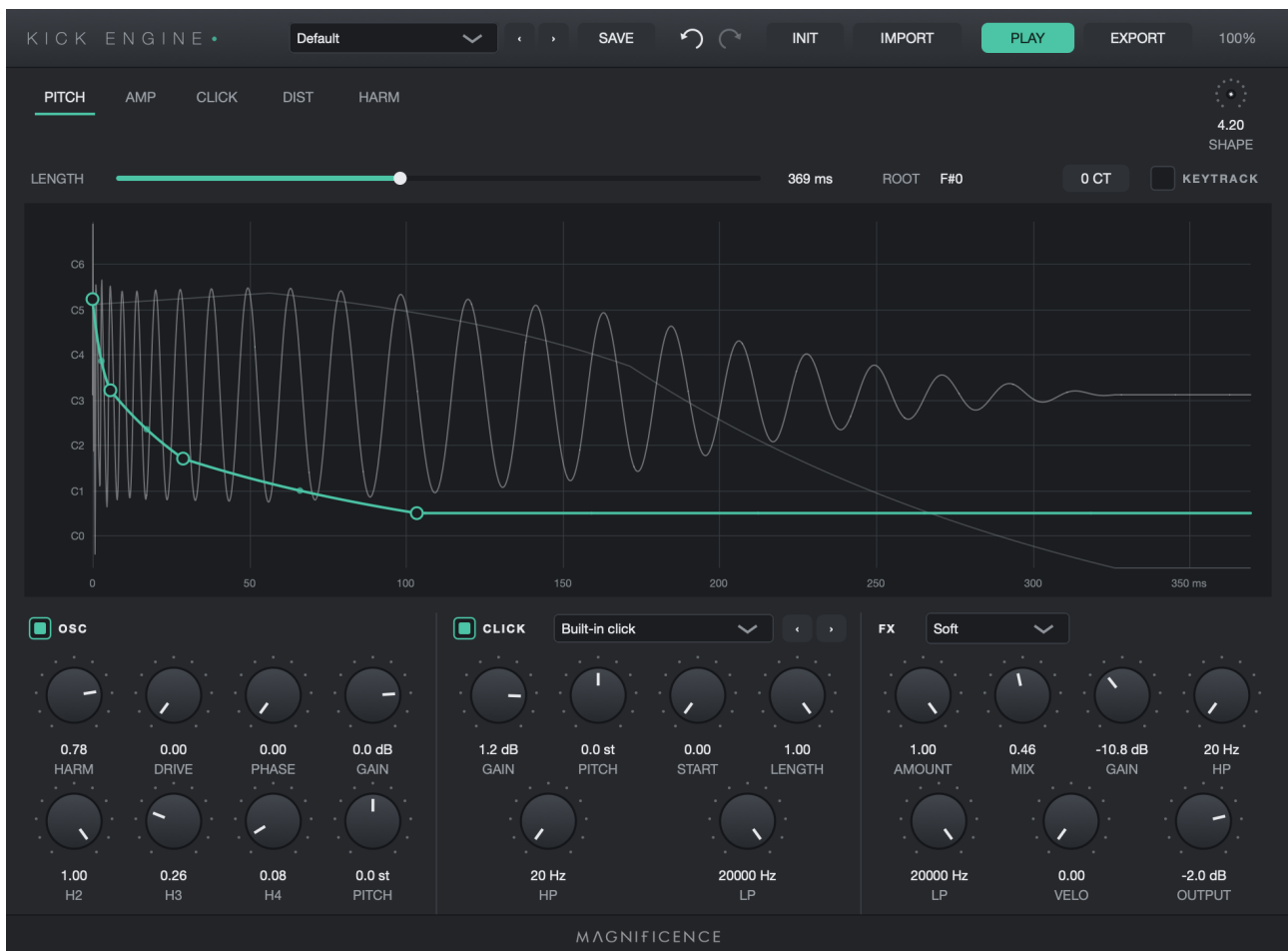
The main window: header, curve editor, and the OSC / CLICK / FX sections.
